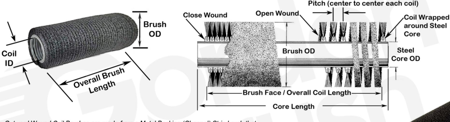
Outward Wound Coil Brushes are made from a Metal Backing (Channel) Strip brush that is formed into a "Coil or Spiral" shape. It can be mounted to a Shaft or Steel Tube Core.
